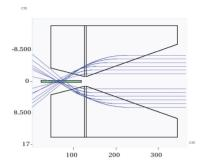
Figure 1: Schematic drawing of  $\nu$ STORM magnetic horn and target(middle rod). Protons hitting the target from left.
