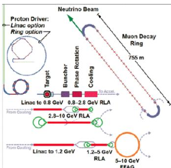
Figure 8: The layout of a Neutrino Factory[28].
