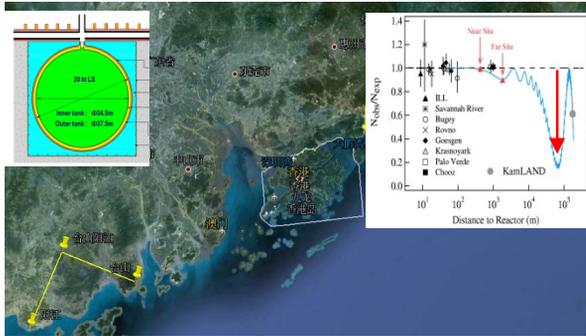
Figure 5: The experimental plan using reactor neutrinos for the mass hierarchy.
