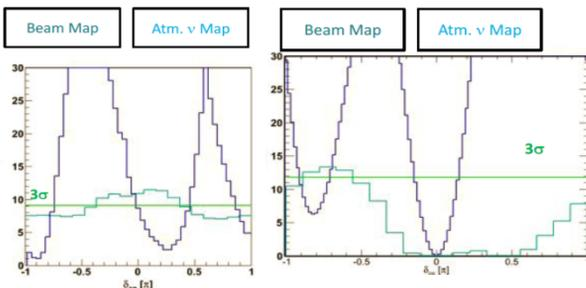
Figure 6: Sensitivity of HyperK to the mass hierarchy and CP phase, using atmospheric neutrinos and accelerator neutrino beams[20].
