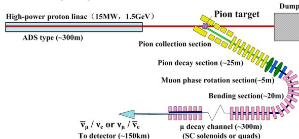
Figure 9: The layout of the neutrino beam from muon decays.
