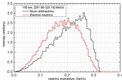
Figure 10: The energy spectrum of neutrinos from the muon decay pipe.
