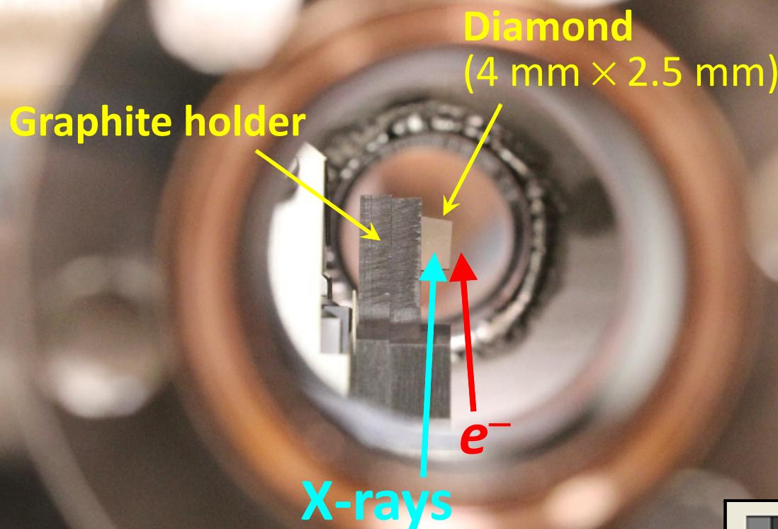
Crystal is high quality 110-μm thick type-IIa diamond crystal plate with (004) lattice orientation.
