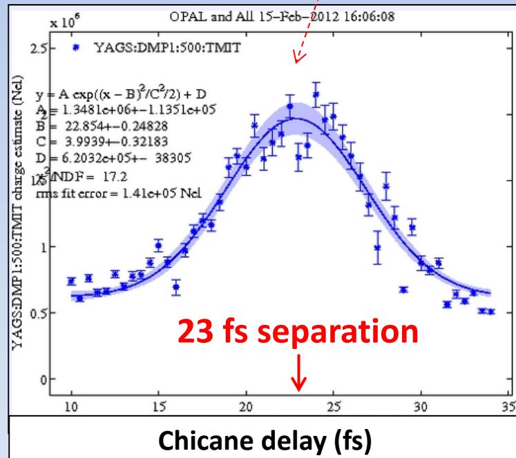
measured rms pulse duration is 3-4 fs
