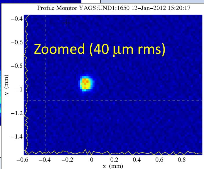
Intensity jitter here is 100% (not saturated and only narrow band is reflected)
