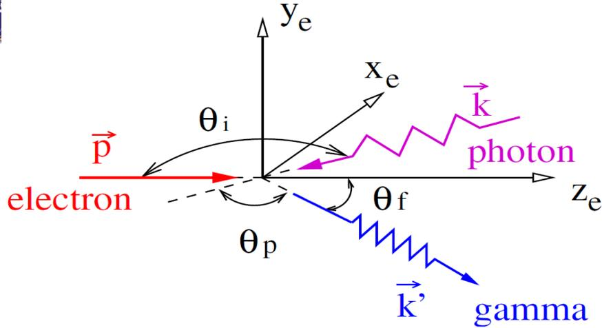
$$E_\gamma \equiv \hbar\omega' = \frac{\hbar\omega(1 - \beta \cos \theta_i)}{1 - \beta \cos \theta_f + \frac{\hbar\omega}{\mathcal{E}_e}(1 - \cos \theta_{ph})}$$
