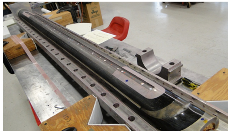
Coil after impregnation with epoxy
