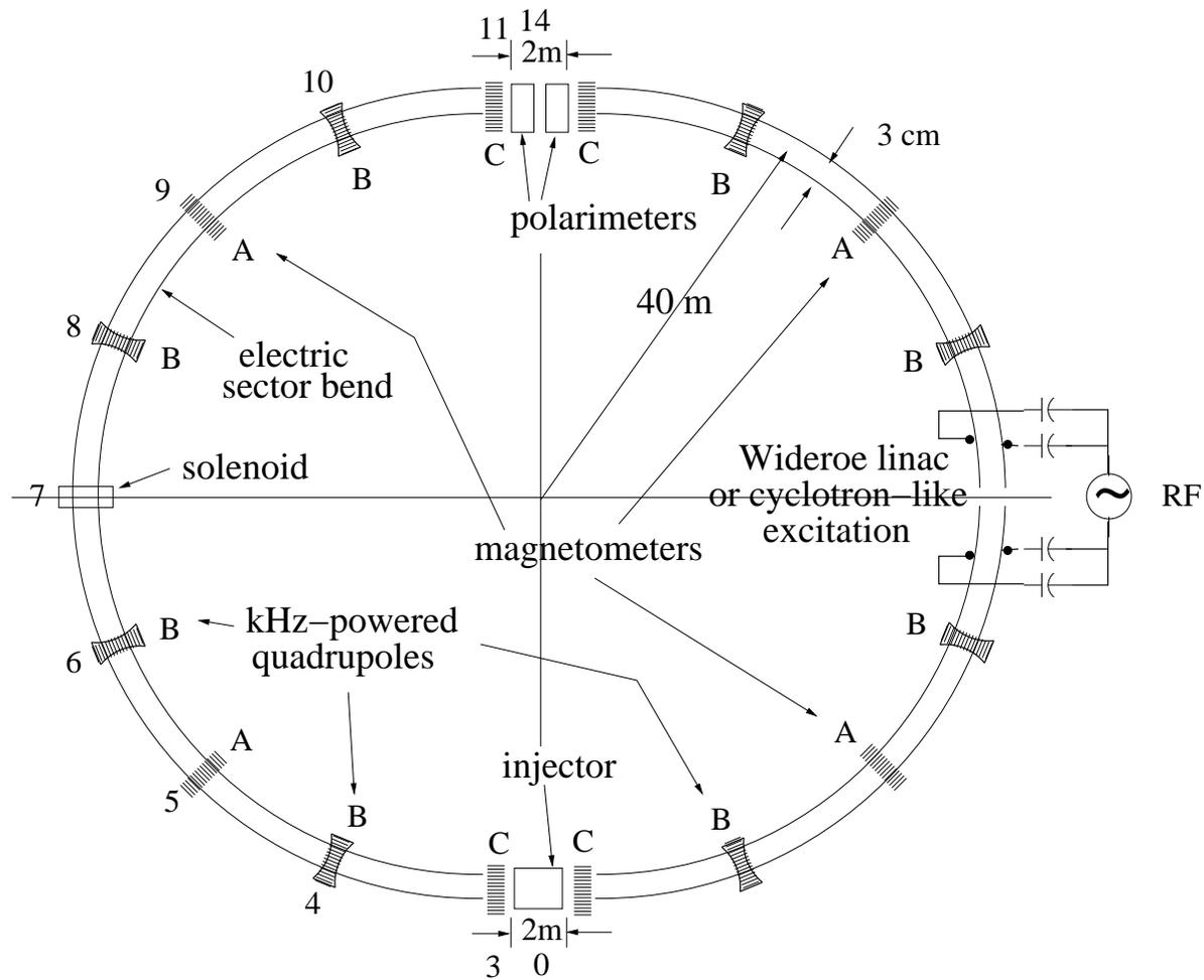
Figure 1: A (very) weak focusing all-electric lattice (BNL proposal) for measuring the electric dipole moment of the proton. There are counter-circulating proton beams.
