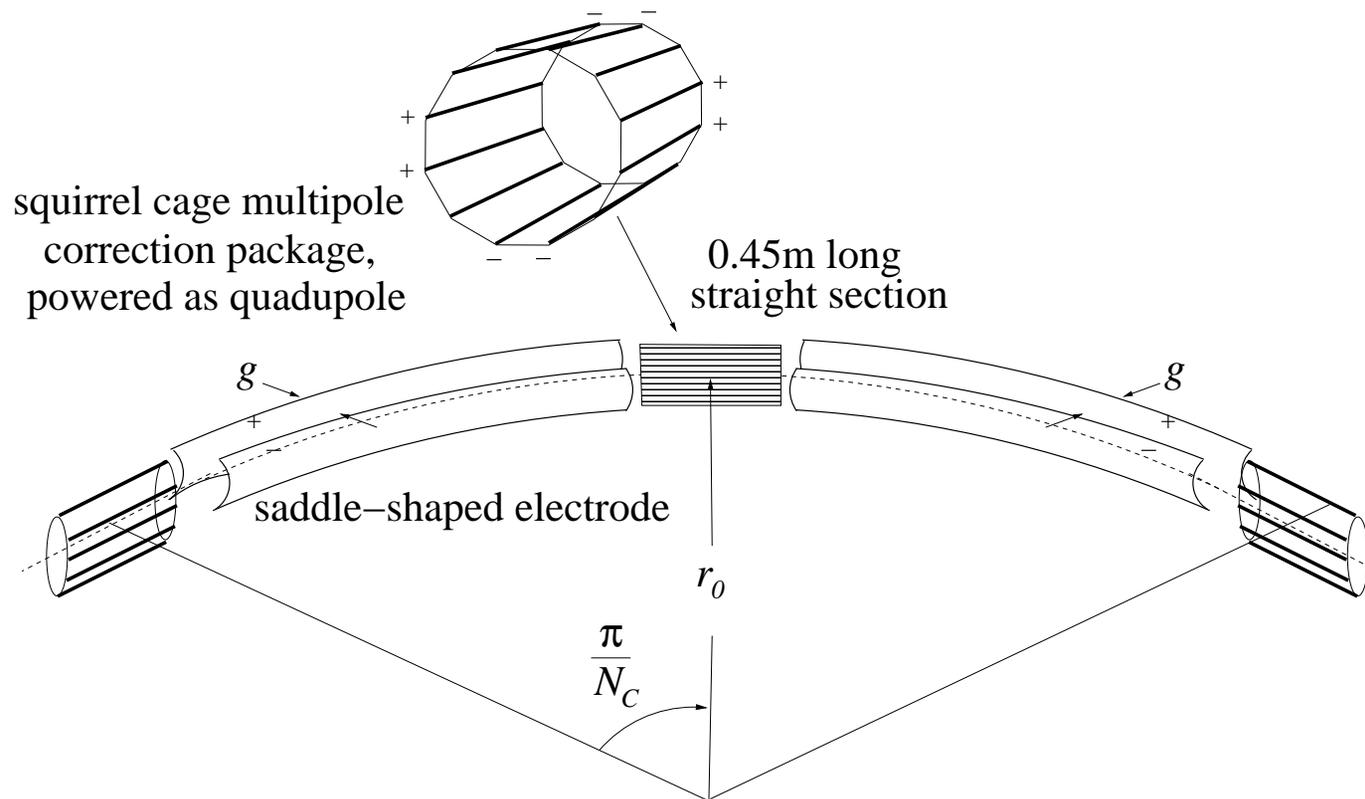
Figure 2: One cell of all-electric proton EDM lattice, with electrodes shaped for design field index  $m$ .
