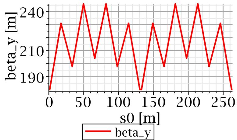
Figure 3: Plots of  $\beta$  functions of proton EDM lattice.  $\beta_y$  is *necessarily* very large, since  $Q_y$  has to be small.
