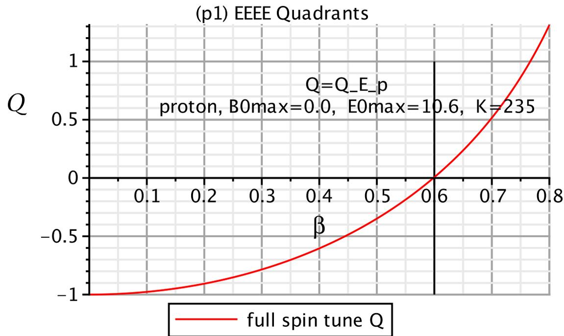
Figure 4: Velocity dependence of (magnetic) spin tune  $Q$  for protons in all-electric lattice. The spin is “globally frozen” for  $\beta=0.6$ . The spin is locally, but not globally, frozen for  $\beta=0.76$ , where  $Q$  is an integer other than zero.
