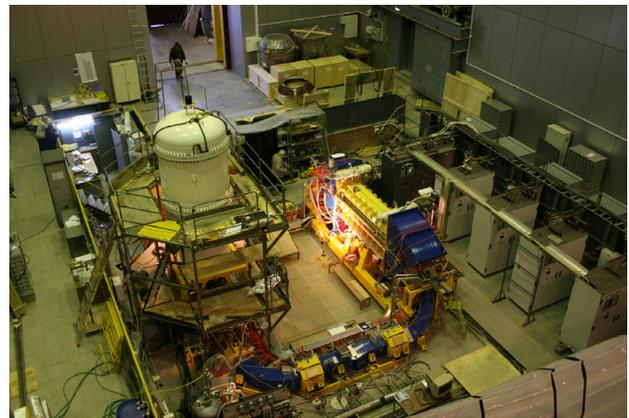
Figure 11: COSY cooler under commissioning at BINP.
