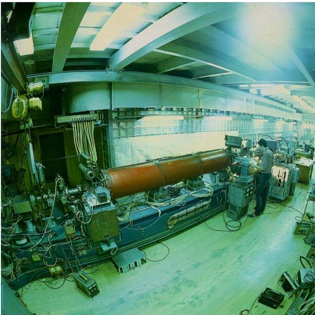
Figure 2: Test bench for direct measuring cooling force.
