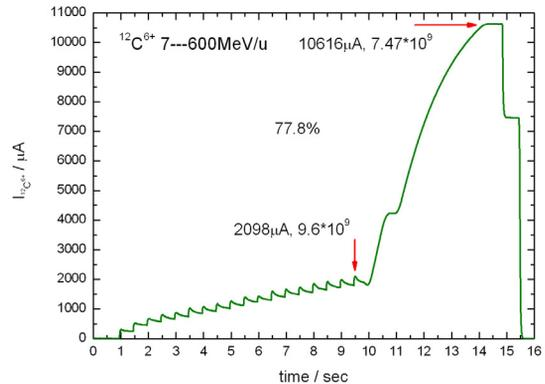
Figure 7: CSRm accumulation C beam and acceleration t0 600 MeV/u.
