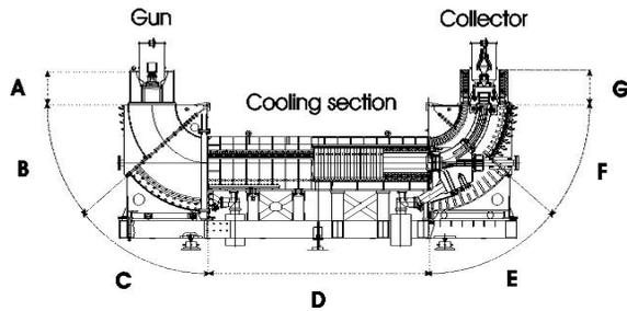
Figure 8: Schematic diagram of the LEIR cooler. A is the gun solenoid with the longitudinally varying magnetic field for expanding the electron beam radius, B and F are small 45-degree toroids with electrostatic deflecting plates, C and E are the main toroids for the joint ion and electron beams, D is the cooling straight section, and G is the collector solenoid.
