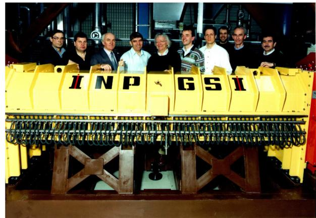
Figure 4: The electron cooler for SIS-18.
