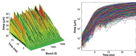
Figure 5. Simulated vertical beam ion instability in DRFS configuration. The vertical instability growth time is  $0.91 \text{ ms}$ .
