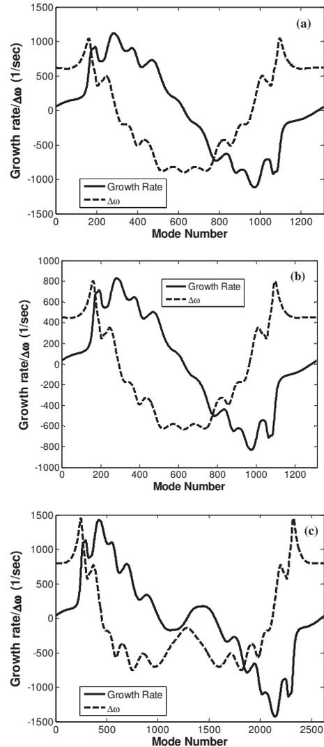
Figure 3. Calculated growth rate and frequency shift due to ions for different beams (a) KCS; (b) DRFS; (c) FP upgrade.
