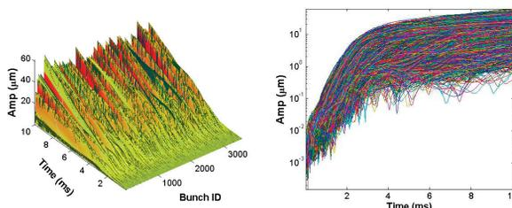
Figure 6. Simulated vertical beam ion instability in FP upgrade configuration. The vertical instability growth time is  $0.40 \text{ ms}$ .
