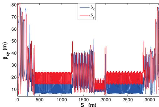
Figure 1. Betatron functions of the DTC02 lattice
