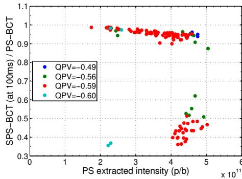
Figure 1: Ratio of the SPS intensity at 100 ms to the PS extracted intensity for different settings of the vertical chromaticity knob QPV.
