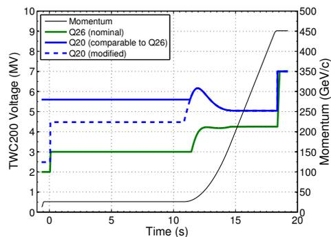
Figure 3: Momentum and 200 MHz voltage program along the cycle for the Q26 and Q20 optics, together with the modifications mentioned in the text.
