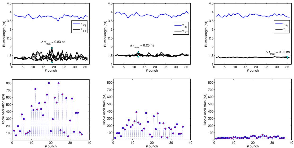
Figure 4: Bunch length (top) and bunch position (bottom) oscillations at flat top for the bunches of single batch 50 ns LHC beam. Columns correspond to Q26 (left), Q20 with comparable RF settings (middle) and Q20 after optimization (right).
