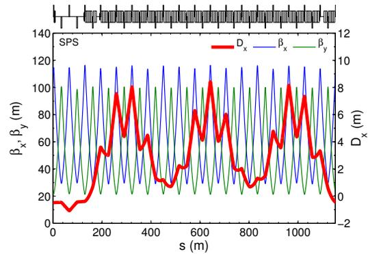
Figure 2: SPS optics with split tunes. Small vertical beta functions are obtained keeping the vertical tune at its nominal value, while the reduced horizontal tune yields low  $\gamma_t$ .
