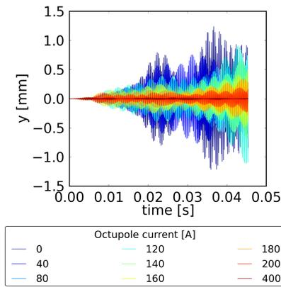
Figure 3: The vertical coherent motion under the influence of electron clouds at an energy of 450 GeV for different octupole currents.
