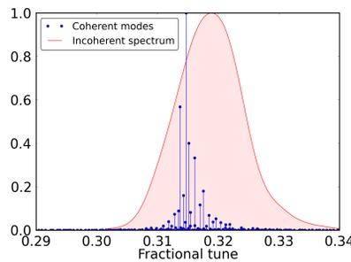
Figure 4: The coherent vs. incoherent mode spectrum. The large overlap indicated there are sufficient resonant particles contributing to Landau damping.
