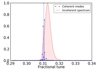
Figure 6: The coherent vs. incoherent mode spectrum. The incoherent spectrum is shifted away from the coherent spectrum and is too narrow to sufficiently cover the coherent modes.
