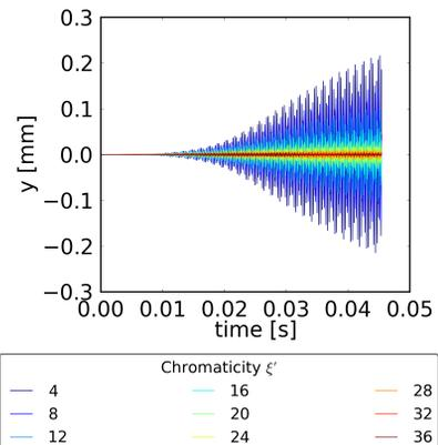
Figure 2: The vertical coherent motion under the influence of electron clouds at an energy of 3.5 TeV for different chromaticities.
