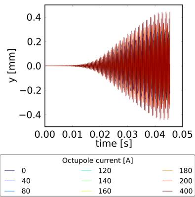
Figure 5: The vertical coherent motion under the influence of electron clouds at an energy of 3.50 TeV for different octupole currents.
