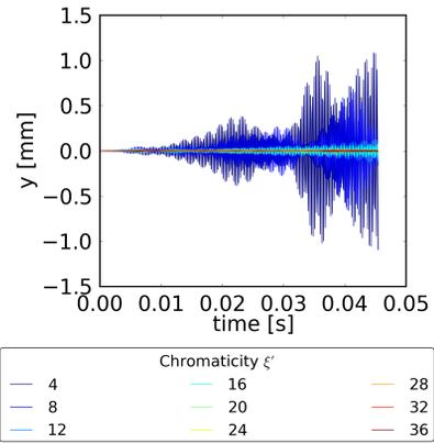
Figure 1: The vertical coherent motion under the influence of electron clouds at an energy of 450 GeV for different chromaticities.
