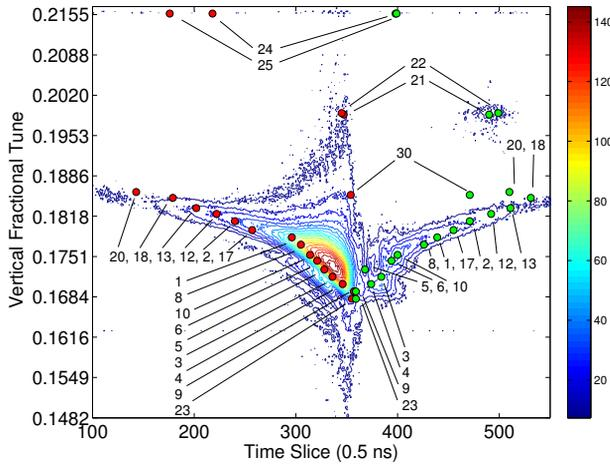
Figure 2: (Color) Betatron tune along the bunch and the greatest strength location for the first 30 ICs, some of which lie outside the plot boundary. The contour plots  $\text{fft}(x)$  along turn for each time slice. The red and green circles mark the leading and trailing edge greatest strength locations respectively with IC number indicated by numeric labels. The beam profile peak is located at time slice 350.
