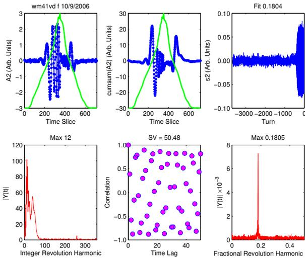
Figure 1: (Color) Typical betatron IC resulting from ICA of the difference signal for a single-turn kick.
