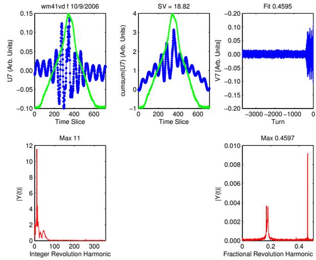
Figure 3: (Color) Typical betatron PC resulting from PCA of the difference signal for a single-turn kick.
