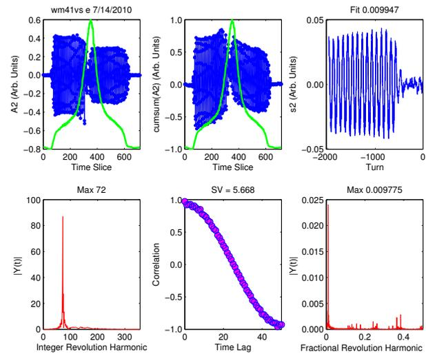
Figure 6: (Color) 201.25 MHz IC resulting from ICA of the sum signal when the revolution frequency is near an integer subharmonic of the linac frequency.
