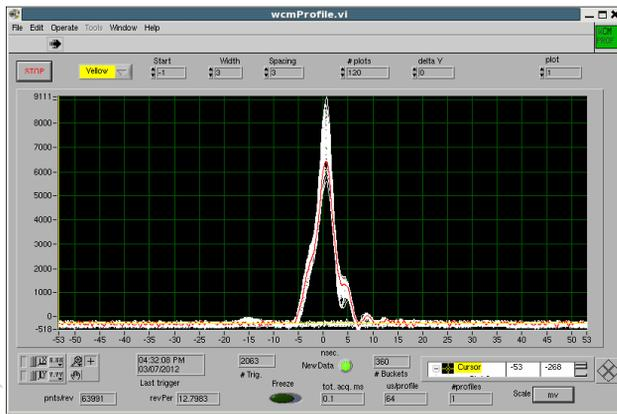
Figure 2: Wall current monitor profiles of 109 Yellow bunches at injection during high intensity tests. At an average intensity of  $2 \cdot 10^{11}$  protons per bunch and an average RMS bunch length of  $\sigma_s = 2$  nsec, the average of the bunch peak currents reaches 7.5 A.
