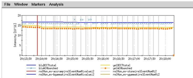
Figure 5: Total beam intensity of six bunches in each ring during a high intensity test ramp.
