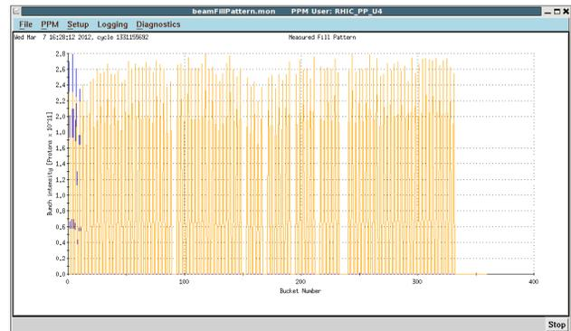
Figure 3: Yellow bunch-by-bunch fill pattern during high intensity tests at injection. The average intensity of the 109 bunches reaches  $2.6 \cdot 10^{11}$  protons per bunch.
