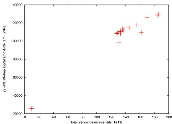
Figure 1: Loss rate measured at dump beam loss monitor y9-lm3.10-dmp vs. total Yellow beam intensity at time of dump.
