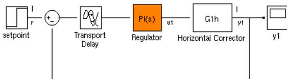
Figure 6: Simulink block for regulator tuning.
