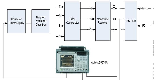
Figure 4: Measurement setup for the fast corrector dynamics.
