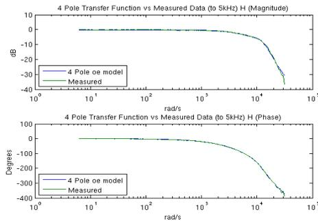
Figure 5: Frequency response from measured data and OE model for horizontal fast corrector at S38.
