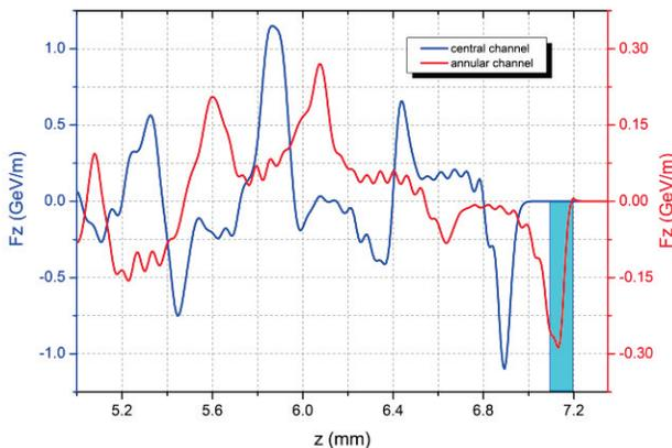
Figure 1: Longitudinal force axial profile at the center of the annular vacuum channel (red line) and at the central channel axis (blue line) in the case of excitation of conventional CDWA [1]. Cyan rectangle shows the
