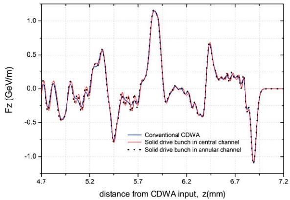
Figure 2: Axial profile of wakefield registered by witness bunch for three regimes of operation of the CDWA: 1) blue line - conventional CDWA; 2) red line - solid drive bunch is in the central channel; 3) black dots - solid drive bunch is in the annular channel.
