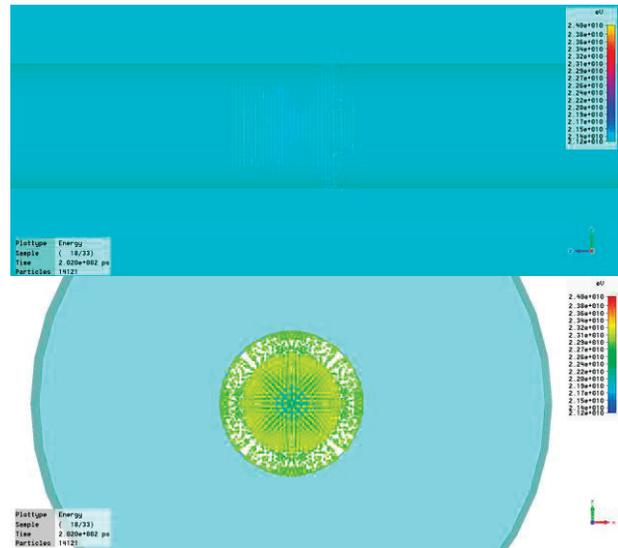
Figure 4: Side (top) and front (bottom) views of the point drive bunch located in the central channel after it has moved 6.1 cm. However, particle losses here are negligible (less 3% of electrons are deposited on inner surface of the inner dielectric tube).
