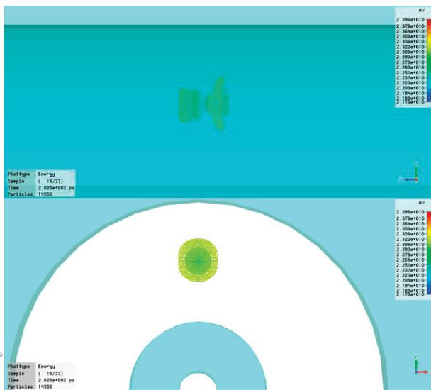
Figure 3: Side (top) and front (bottom) views of the point drive bunch located in the annular channel after it has moved 6.1 cm. Note shape distortion shown at top.
