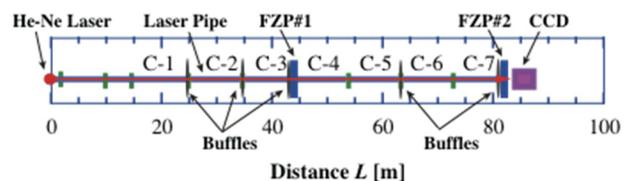
Figure 1: Optical configuration and experimental setup.
