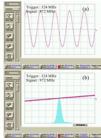
Figure 4: Acceleration frequency in synchronization. The trigger signal in the sampling oscilloscope is the 324 MHz RF and the 972 MHz RF signal is detected. The synchronization of 324 MHz and 972 MHz can be confirmed from (a). (b) shows the wide view. The width of the phase difference using zero cross method is 1.3 fsec in rms.
