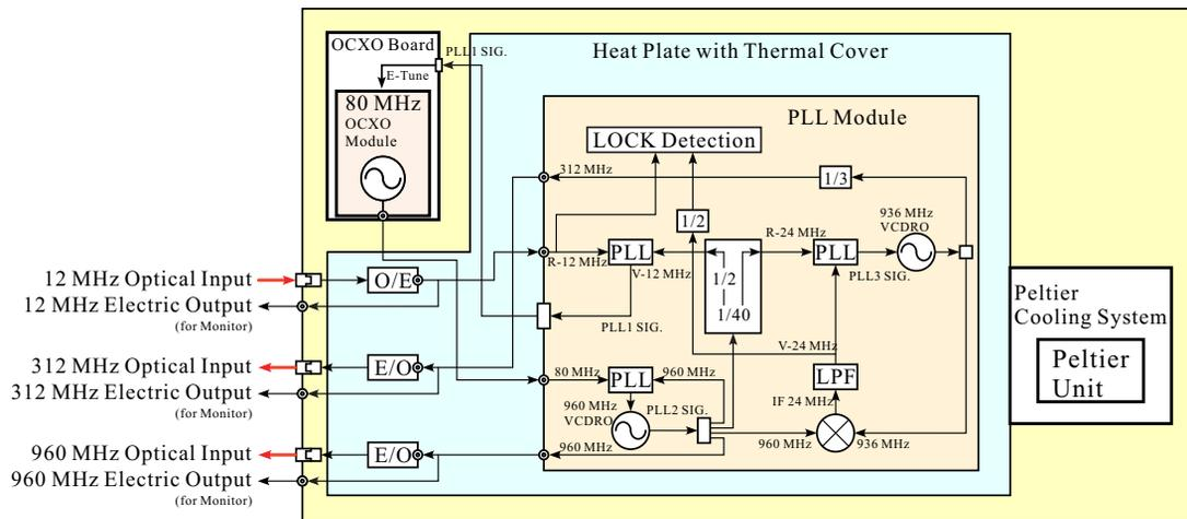
Figure 2: Block diagram of new J-PARC Linac master oscillator. It has the input port of 12 MHz optical signal and the 312 MHz and 960 MHz output signals in synchronization with the input.
