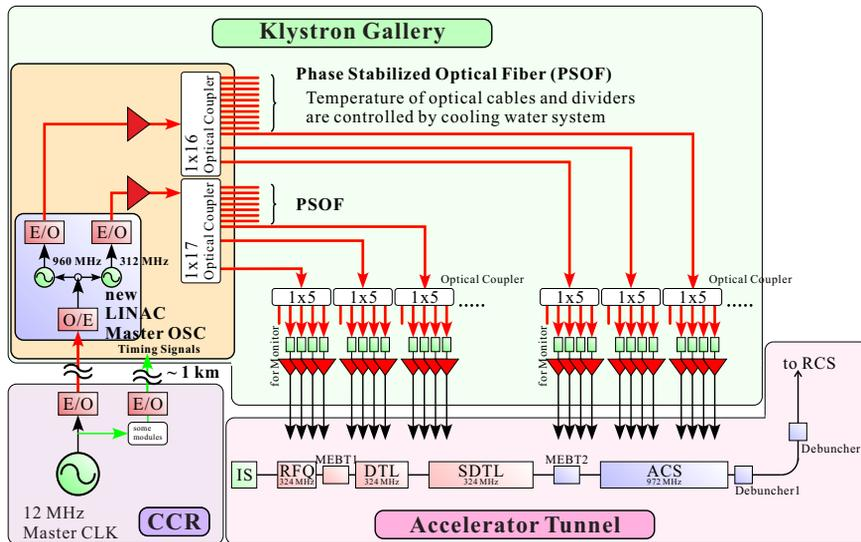
Figure 1: Upgraded J-PARC Linac RF reference distribution system. Two kinds of references, 312 MHz and 960 MHz, can distributed to each control station.
