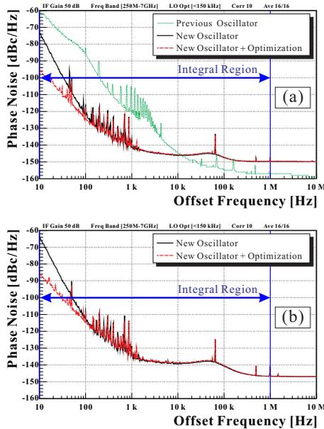
Figure 3: Phase noise of new J-PARC Linac master oscillator. (a) and (b) show the 312 MHz and 960 MHz output signals, respectively. The green line represent and the 312 MHz and 960 MHz output signals in synchronization with the input.
