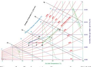
Figure 3: Psychometric diagram of HAVC commissioning with run-around coils.
