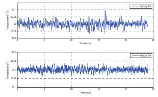
Figure 5: Highly precise control of temperature with runaround coils.
