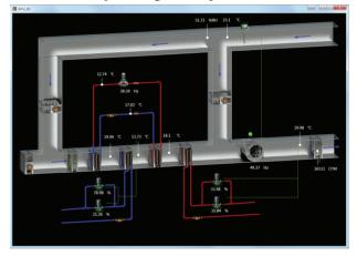
Figure 4: Graphic view of online monitor of the HVAC system.
