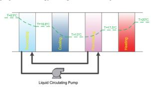
Figure 2: Proposed AHU with run-around coils.
