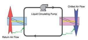
Figure 1: Scheme of run-around system to recover heat and moisture.
