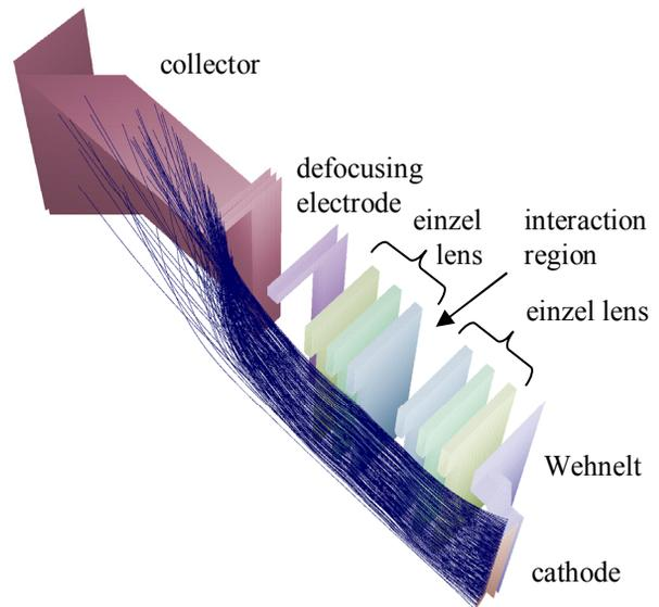
Figure 5: Example for 3D-simulations for the transverse electron target.
