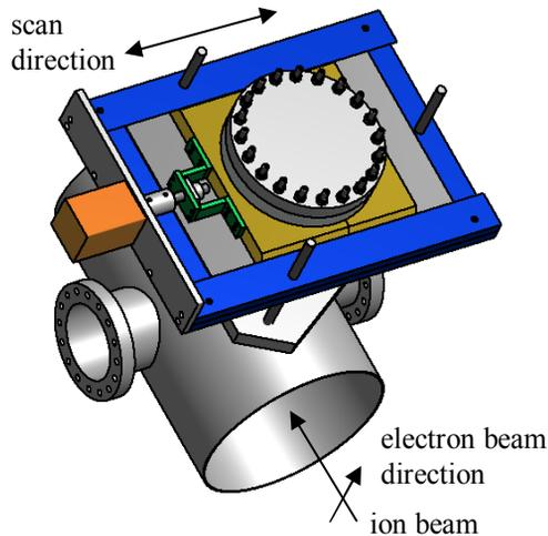
Figure 4: Manipulation system of the transverse electron target.
