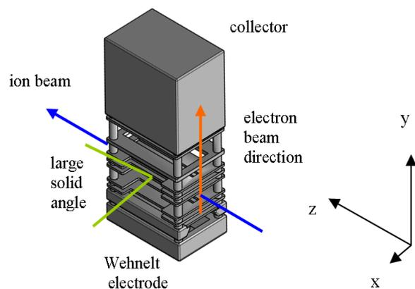
Figure 3: Schematic drawing of the transverse electron target (preliminary).
