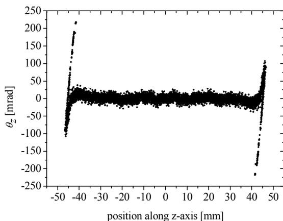
Figure 2: Divergence angle of the electron beam in the interaction region from 3D-simulations with a cathode temperature of  $T_c = 0.1$  eV.
