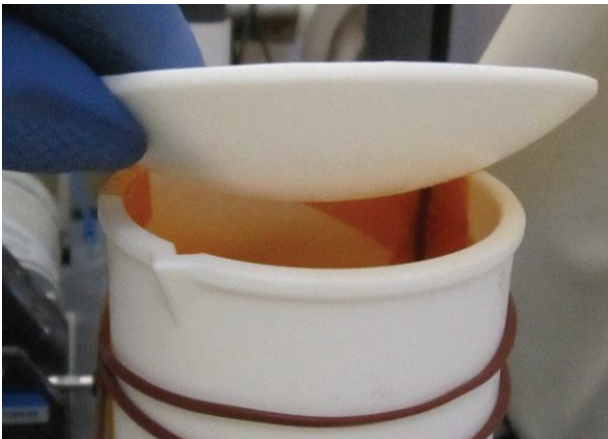
Figure 2: Orange nitric oxide vapors being formed during the reaction between BCP and niobium.
