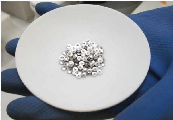
Figure 1: Niobium pellets used during heat of reaction experiments.
