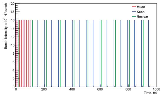
Figure 3: Beam structure for 3 GeV program
