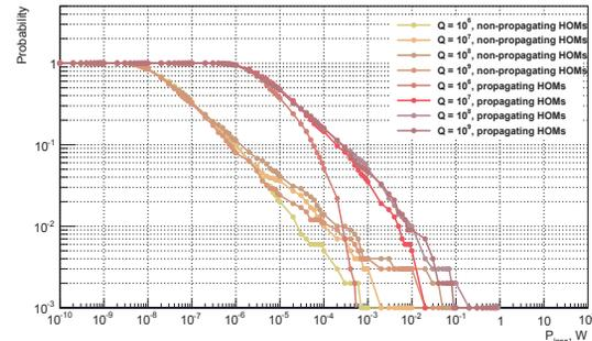
Figure 5: Power loss in 650 MHz cavities for 3 GeV beam structure
