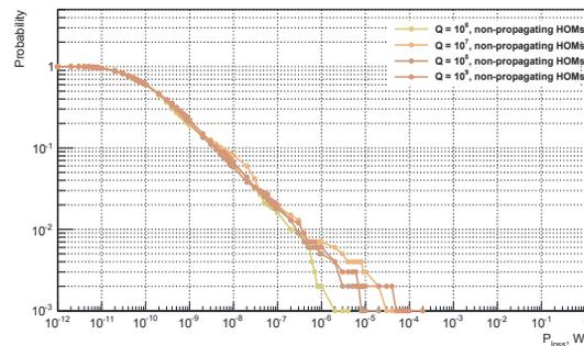
Figure 8: Power loss in SSR1 cavities for 3 GeV beam structure
