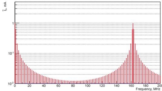
Figure 6: Beam spectrum of Muon Collider pulses
