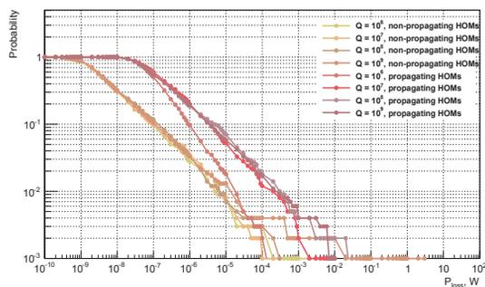
Figure 7: Power loss in 650 MHz cavities for Muon Collider beam structure
