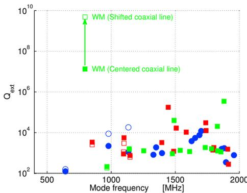
Figure 4:  $Q_{ext}$  of the 45° antenna design.
