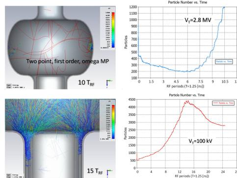
Figure 9: (Top) electron trajectories and population after 10 RF periods at high deflecting voltage (2.8 MV) and (bottom) after 15 RF periods at low deflecting voltage (100 kV).
