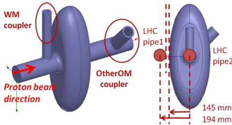
Figure 1: Perspective view of the cavity with couplers encircled (left); View in beam direction of the cavity with spatial constraints highlighted (right). Maximum extension 292x729 mm.
