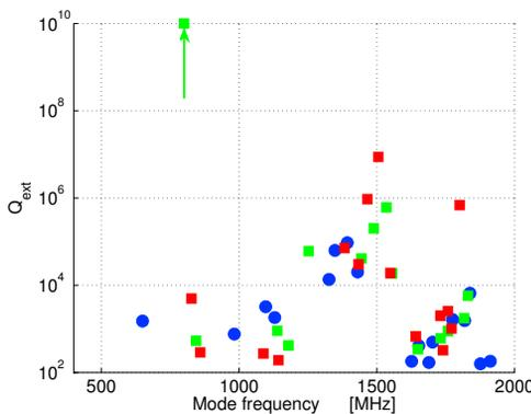
Figure 5:  $Q_{ext}$  of the notch filter design with very high rejection of the WM, larger than  $10^{12}$  (out of scale).
