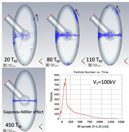
Figure 8: Electron trajectories and population at 4 different time and at low deflecting voltage (100 kV).
