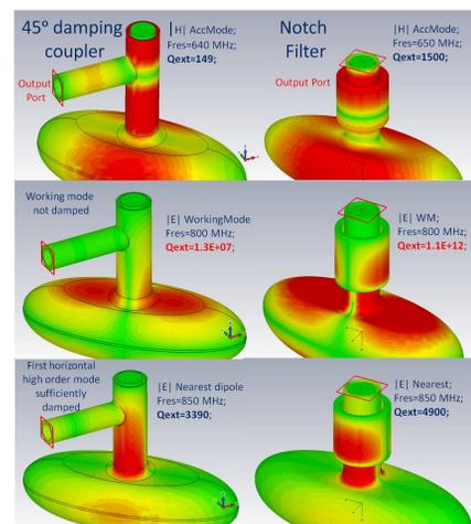
Figure 3: (Top) damping schemes for the fundamental mode and (center/bottom) for the first two dipole modes.
