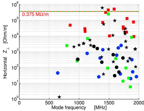
Figure 7: Notch filter coupler: longitudinal and transverse beam impedances.
