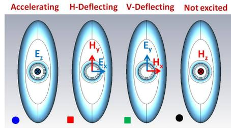
Figure 2: (From left to right) pure accelerating, horizontal and vertical deflecting and not excited modes. Trapped mode will be represented by black stars.
