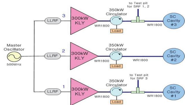
Figure 4: PLS-II RF system of phase-III, adding one more SRF station from phase-II (2014~).
