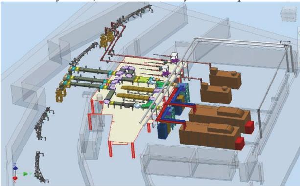
Figure 1: PLS-II RF system [phase-I].
