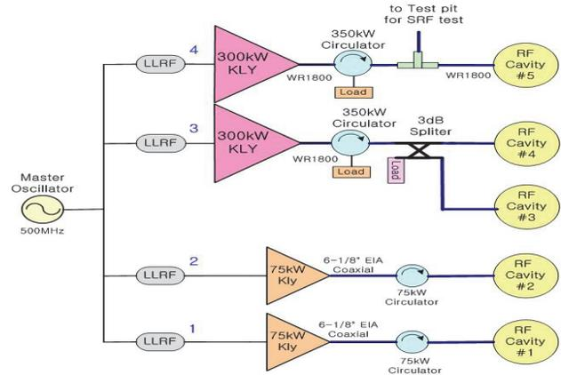
Figure 3: PLS-II RF system of phase-I (~2012).
