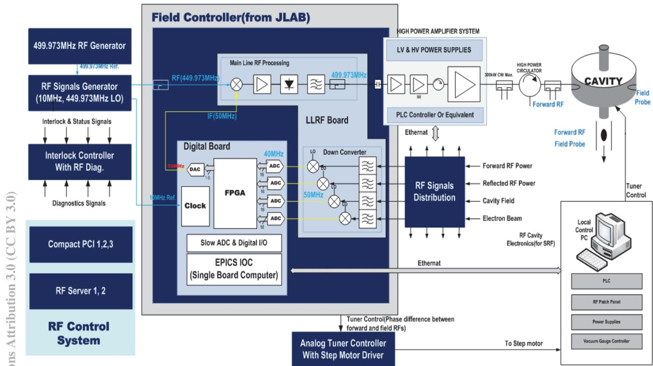
Figure 5: Block diagram of PLS-II RF system with LLRF control.
