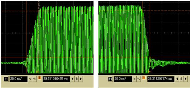
Figure 6: Detail of rising and falling edges, 20ns/div. 10-90% risetime = 14.3ns, falltime = 8.3ns.
