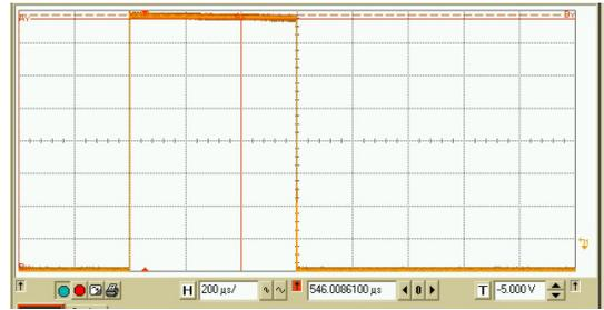
Figure 8: Amplitude stability. Amplitude droop through pulse = 1.3%. Spread over 1000 pulses = 0.85%
