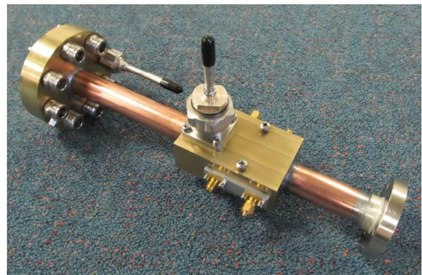
Figure 3: The 15kW 6:1 radial combiner / dual directional coupler assembly.
