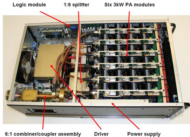
Figure 1: Internal layout of the power amplifier chassis (15kW, 324MHz). The amplifier output stage operates at approximately 68% efficiency, and is fan cooled.
