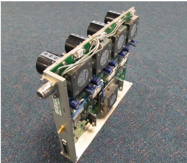
Figure 2: Internal layout of the 3kW power amplifier module, showing input and output circulators and quadrature hybrids.
