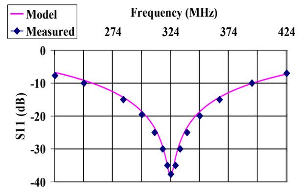
Figure 4: Modelled and measured return loss of the 6:1 combiner / dual directional coupler assembly.
