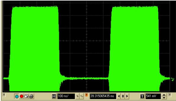
Figure 5: 30kW "micro-pulses", 100ns/div.
