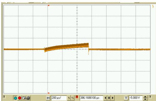
Figure 7: Phase stability. Vertical scale 1.5 $^{\circ}$ /div. Phase change through pulse = 0.75 $^{\circ}$ , phase spread over 1000 pulses = 0.5 $^{\circ}$ p-p.
