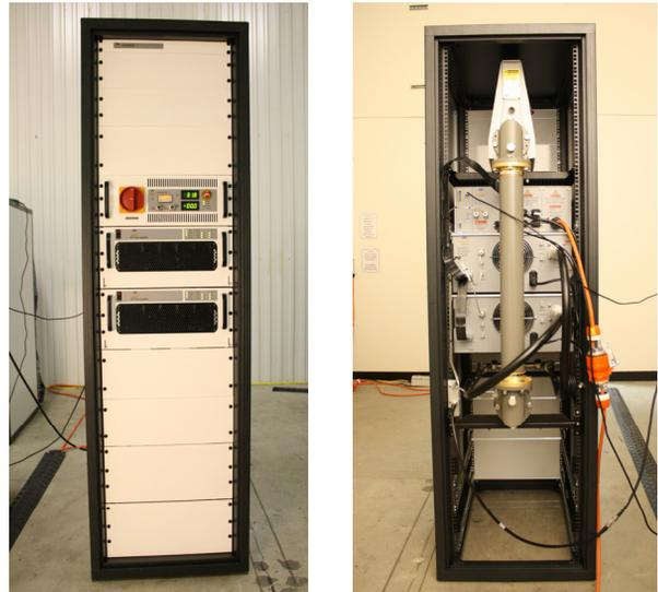
Figure 9: Front and rear views of the amplifier rack. The empty space at the bottom of the rack allows for additional amplifier units for a power upgrade.
