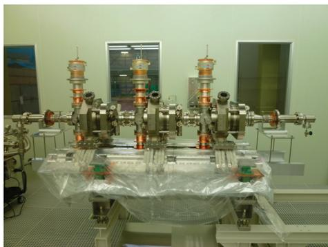
Figure 8: String assembly of three 2-cell cavities with six input couplers in a class-10 clean room.
