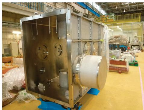
Figure 9: Vacuum vessel for cERL injector cryomodule.
