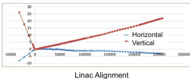
Figure 9: Linac tuning. It was 2.6 cm down in the middle and, then moved up (Linac is no longer linear).
