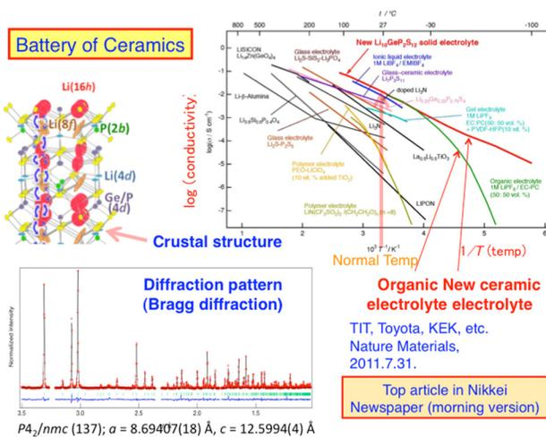
Figure 4: New ceramic battery observed by neutrons.
