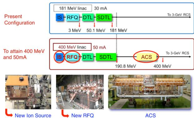
Figure 10: 400 MeV Linac which is under construction.
