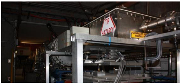
Figure 5: Collimator wakefield chamber test allows an exchange of collimators and adjustment of jaw aperture.
