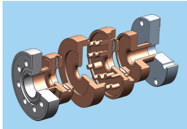
Figure 1: Expanded three-quarter view of solid model of elliptical-rod PBG structure, showing two coupling cells and central PBG cell. Power is coupled in from the left.
