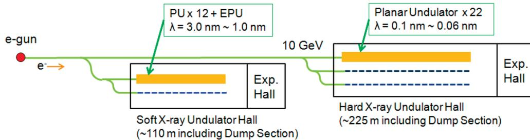
Figure 4: Layout of the current design of the PAL-XFEL undulator.
