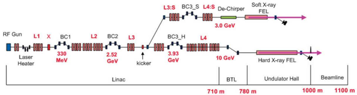
Figure 3: Layout of the current design of the PAL-XFEL linac.
