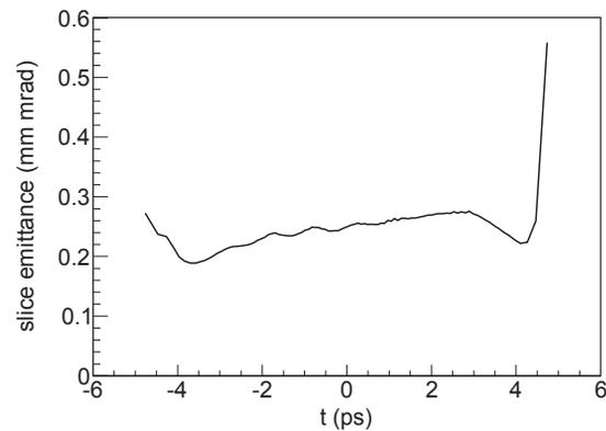
Figure 4: Rms slice emittance of a 200 pC bunch at the injector end.
