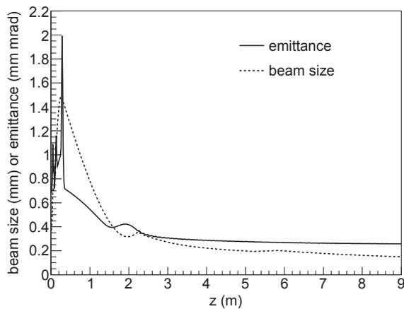
Figure 3: Normlized rms transverse emittance and rms beam size of a 200 pC bunch vs. distance from the cathode.
