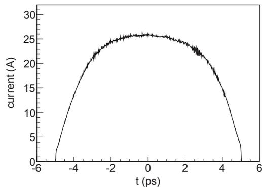
Figure 5: Current profile of a 200 pC bunch at the injector end.
