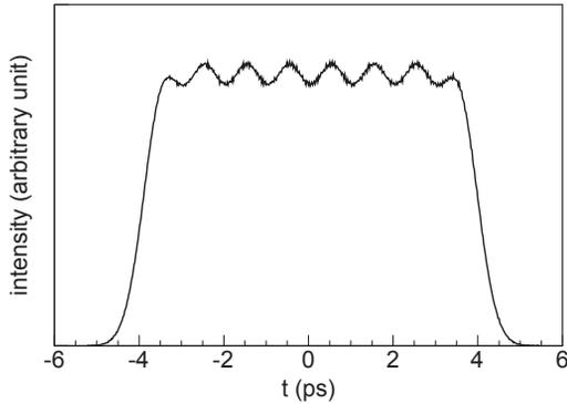
Figure 2: Longitudinal profile of a drive laser pulse. Eight Gaussian pulses with a 0.45 ps rms length are stacked.
