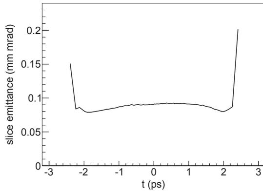
Figure 6: Rms slice emittance of a 20 pC bunch at the injector end.
