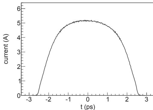
Figure 7: Current profile of a 20 pC bunch at the injector end.
