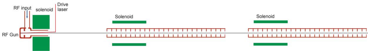
Figure 1: Layout of the injector consisting of an RF photocathode gun, focusing solenoids, two accelerating sections, and a laser heater system (not shown here).
