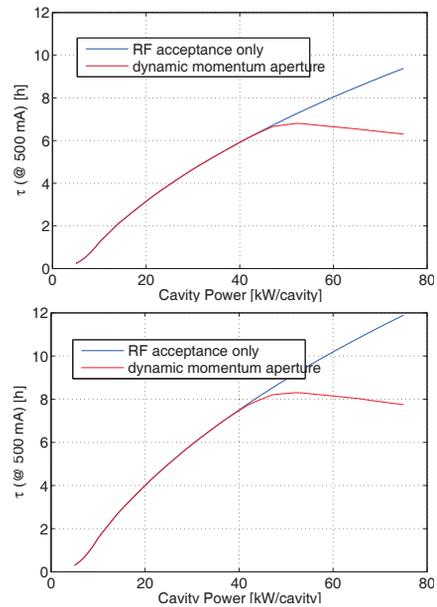
Figure 5: Touschek lifetime with (top) skew quads off and (b) skew quads on.
