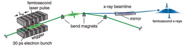
Figure 1: Schematic of a femtosecond slicing beamline [2].
