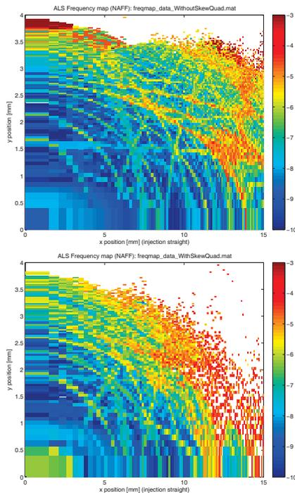
Figure 4: Dynamic aperture with (top) skew quads off and (bottom) skew quads on.
