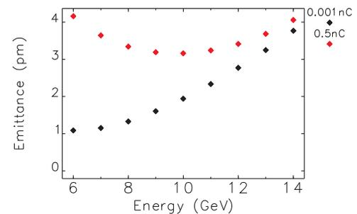
Figure 4: Emittance as a function of beam energy for two values of bunch charge, assuming full coupling.
