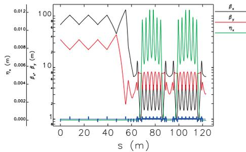
Figure 2: Typical lattice functions, showing half of the long straight section along with two arc cells.
