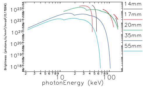
Figure 6: Curves of brightness in ph/s/mm<sup>2</sup>/mrad<sup>2</sup>/0.1%BW for various undulators.
