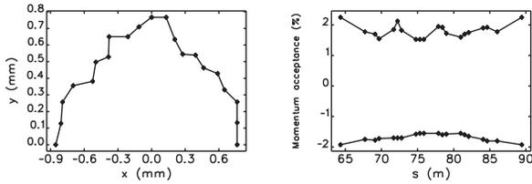
Figure 5: Preliminary MOGA optimization results, showing the dynamic acceptance (left) and the momentum acceptance (right) for one arc cell.
