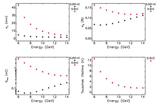
Figure 3: Collective effects as a function of beam energy for two different levels of bunch charge.
