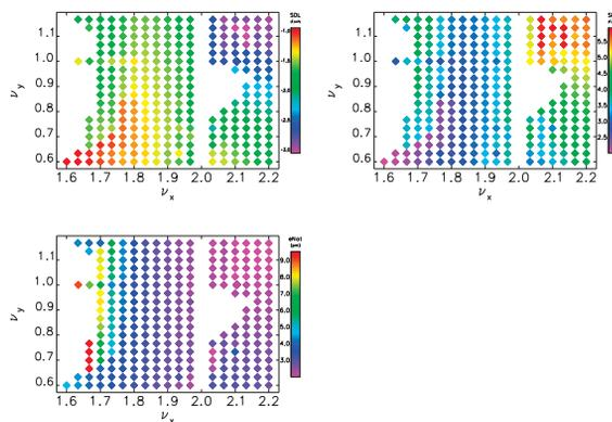
Figure 1: Integrated SD and SF sextupole strengths (top left and right) in  $1/m^2$  and natural emittance (bottom right) in pm as a function of cell tunes at 9 GeV.
