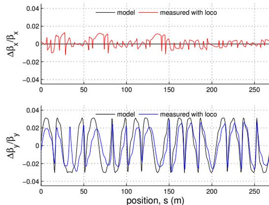
Figure 5: The horizontal (top) and vertical (bottom) beta beating introduced by the superconducting wiggler: the model values are compared with the measured ones.
