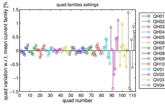
Figure 3: Quadrupole change applied to symmetrize the ALBA storage ring optics with LOCO.
