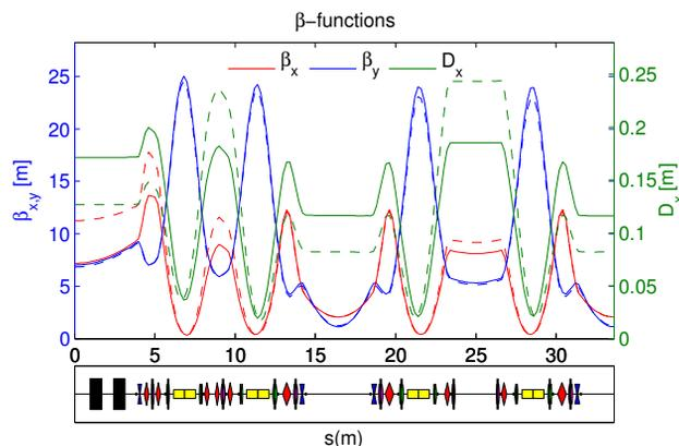
Figure 6: Optic functions comparison between the nominal (dashed lines) and the new optics (continuous lines). One eighth of the machine is shown.
