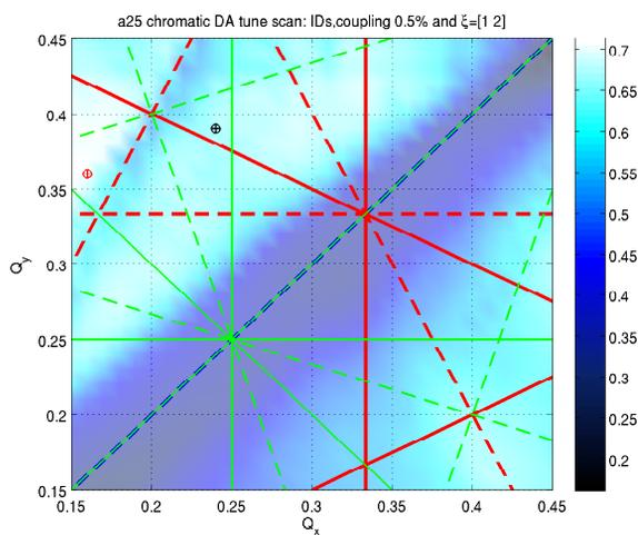
Figure 1: Chromatic dynamical aperture simulations as a function of the working point. The starting working point is represented by a black cross while the new working point is in red.
