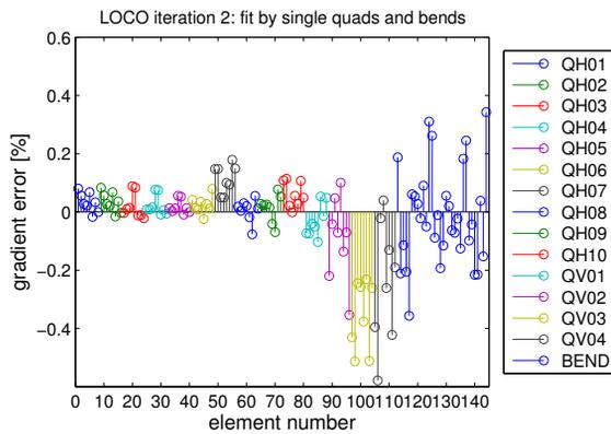
Figure 4: Calibration errors in the 112 quadrupoles and 32 gradient dipoles fit by LOCO.
