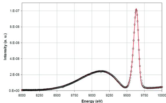
Figure 7: Comparison of the theoretical spectrum to the measured one for one of the in-vacuum undulators. All the nominal settings agree well, with just the energy fitted to 2.998 GeV.
