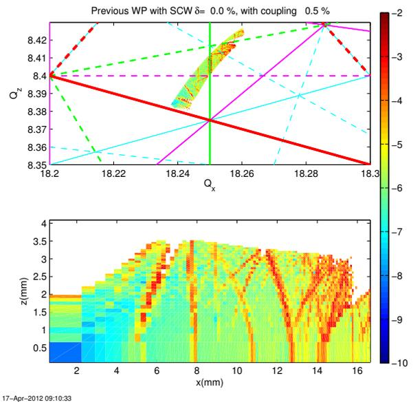
Figure 2: Frequency map for the Alba Lattice including IDs when the tune is close to resonance  $2Q_y + Q_x = 35$ . In this case, the effective elastic lifetime would be considerably reduced.
