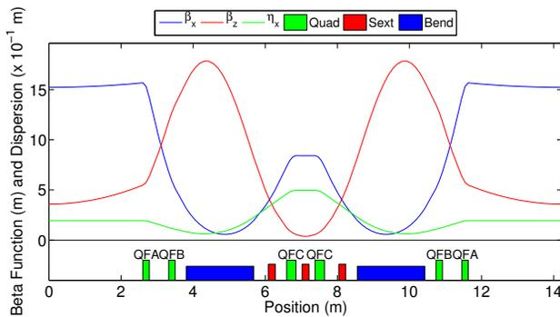
Figure 3: Machine functions for a sample working point in the side region with  $K_a = 3.16 \text{ m}^{-2}$ ,  $K_b = -1.19 \text{ m}^{-2}$  and  $K_c = 2.04 \text{ m}^{-2}$  giving tunes (9.91, 8.08), horizontal dispersion 0.19 m in the straight sections, emittance 17.0 nm and a dynamic aperture of 835 mm<sup>2</sup>.
