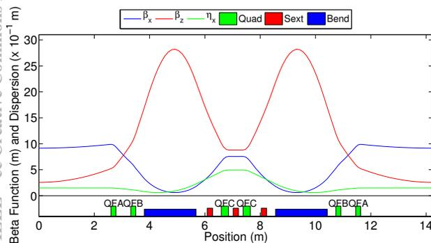
Figure 1: CLS lattice with beta functions ( $\beta_x$  and  $\beta_z$ ) and horizontal dispersion ( $\eta_x$ ) for quadrupole settings  $K_a = 1.968 \text{ m}^{-2}$ ,  $K_b = 1.417 \text{ m}^{-2}$  and  $K_c = 2.045 \text{ m}^{-2}$  giving the nominal tunes (10.22, 4.32).
