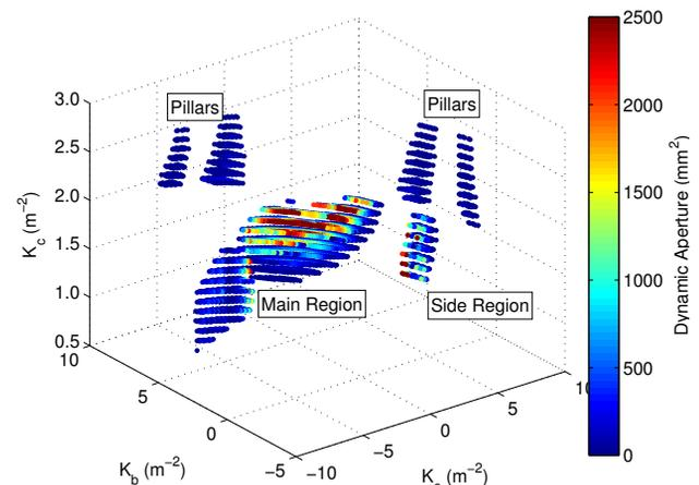
Figure 2: Operating points with emittance less than 30 nm.
