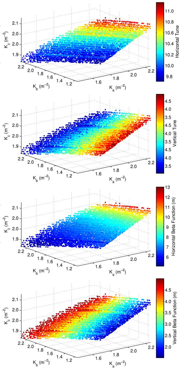
Figure 5: Tunes and center-of-straight beta functions for operating points in the main region with emittance less than 13 nm, center-of-straight vertical beta function less than 5 m and dynamic aperture greater than 100 mm<sup>2</sup>.
