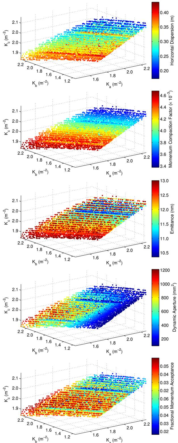
Figure 6: Dispersion, momentum compaction factor, emittance, dynamic aperture and momentum acceptance for operating points in the main region with emittance less than 13 nm, center-of-straight vertical beta function less than 5 m and dynamic aperture greater than 100 mm<sup>2</sup>.
