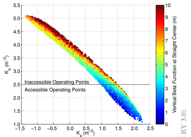
Figure 4: Operating points in the main region with emittance less than 18 nm and dynamic aperture greater than 100 mm<sup>2</sup>; the  $K_c$  axis is suppressed.
