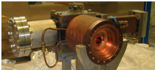
Figure 2: The ALPHA-X S-band RF gun.
