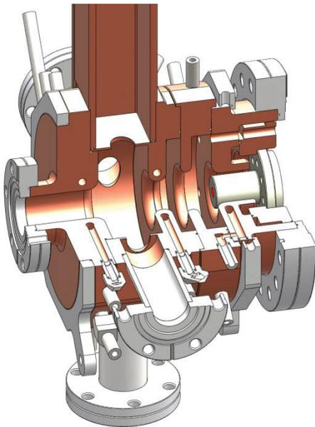
Figure 4: The thermionic RF gun with improved cooling in between the cells and around the cathode, increased coupling and changed geometry of the 1/2 wavelength choke for the cathode mount.
