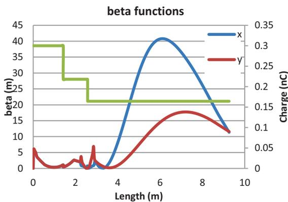
Figure 2: Optical functions and charge for the thermionic gun injection through the first linac. The chopper aperture is placed at 1.4 m from the cathode, the energy filter starts at 2m from the cathode and the linac entrance is at 3.5 m.
