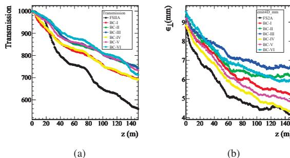
Figure 3: (a) Transmission along the beam-axis. All BC versions achieve as high as 15-20% better transmission than FSIIA; (b) Transverse emittance along the beam-axis. The best cooling overall is obtained by FSIIA and BC-IV.
