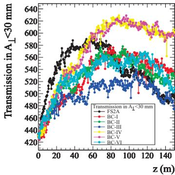
Figure 4: Transmission within  $A_{\perp} < 30$  mm. All BC lattices achieve a better, comparable, or insignificantly lower transmission than FSIIA, at the  $z$ -position where FSIIA has its maximum.
