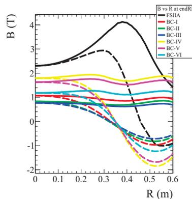
Figure 2: Total (continuous line) and axial (dashed line) magnetic field ( $B_{tot}$ ,  $B_z$ ) along the radius, at the walls of the RF cavities (black: FSIIA; red, green, blue, yellow and cyan correspond to BC-I, -II, -III, IV, V and VI respectively). All BC versions achieve from two to as high as five times smaller  $B_{tot}$  than FSIIA. All BC's have virtually zero  $B_z$  at the iris.
