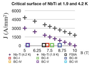
Figure 5: Critical surfaces of Nb-Ti for 1.9 and 4.2 K. All lattices are within the limits of superconducting operation.
