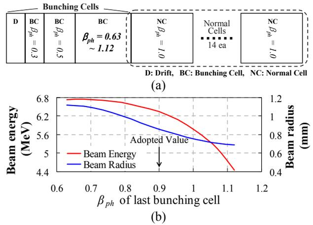
Figure 3: (a) Schematic diagram of the beam dynamics simulation setup for optimizing the configurations of phase velocities in the bunching cells. (b) Variation of beam parameters on  $\beta_{ph}$  of the last bunching cell.
