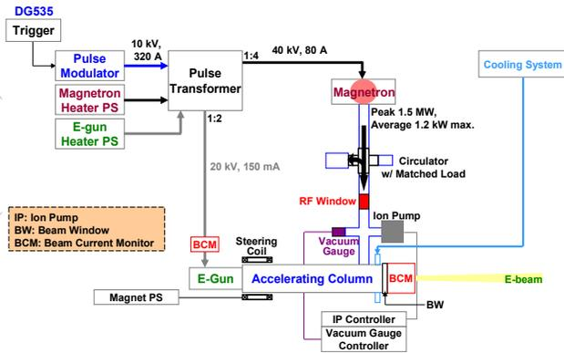
Figure 1: Schematic diagram of the accelerator system.
