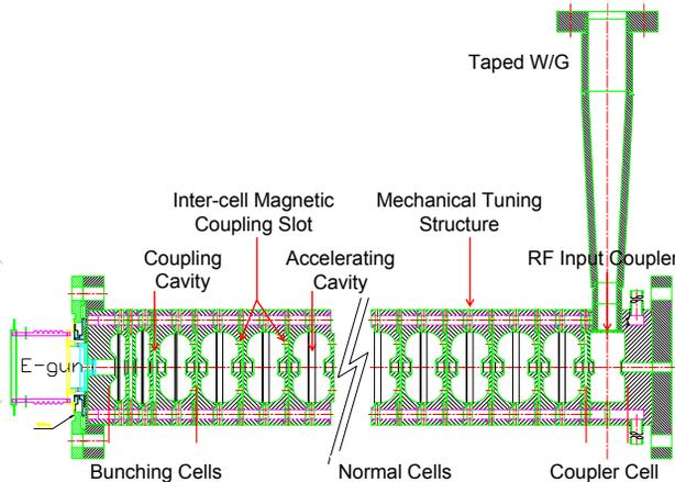
Figure 2: Cross-sectional view of the accelerator structure.
