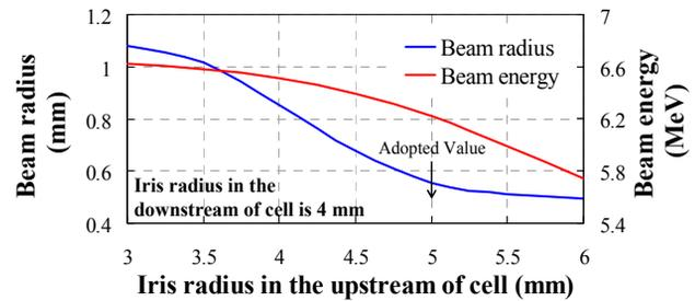
Figure 4: The beam radius and the average beam energy on the iris radius in the upstream of the first bunching cell.
