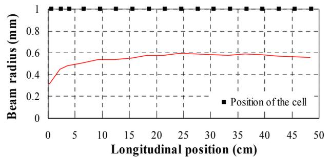
Figure 5: The beam envelop in the accelerating structure.
