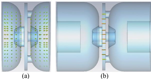
Figure 6: Simulation model to find the resonant frequency for (a): the accelerating cavity, (b): the coupling cavity.
