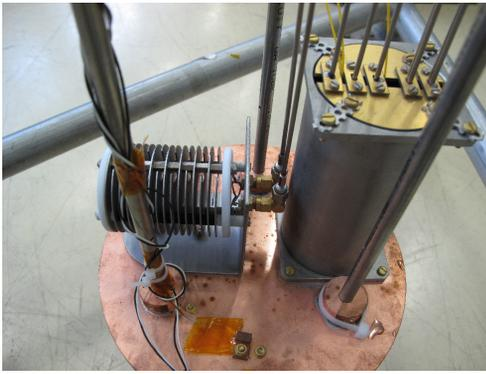
Figure 2: The detectors are mounted on a copper plate, which is lowered into the cryostat. On the left side of the picture is the 10 cm long chamber and on the right is the cylinder containing the semiconductors. Cables with low heat conduction bring out the signal from the detectors to the top of the cryostat.
