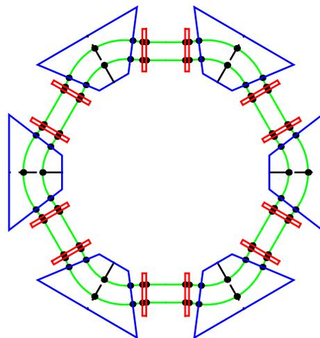
Figure 2: Layout of the 6-cell 0.33–1 GeV FFAG.
