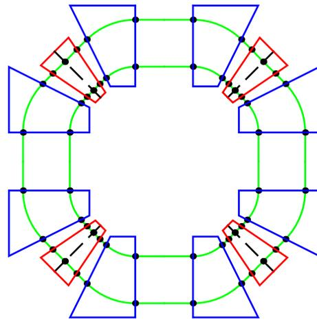
Figure 1: Layout of the 4-cell 0.25–1 GeV FFAG.
