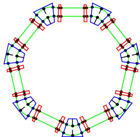
Figure 3: Layout of the 7-cell 0.33–1 GeV FFAG.
