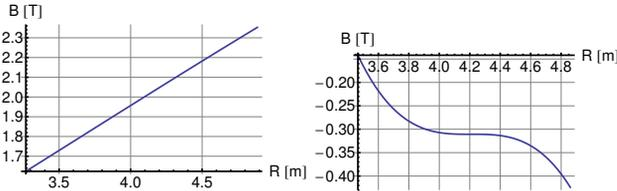
Figure 4: F (left) and D (right) field profiles for the 4-cell 0.25–1 GeV FFAG.
