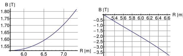
Figure 5: F (left) and D (right) field profiles for the 6-cell 0.33–1 GeV FFAG.
