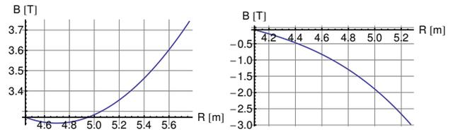
Figure 6: F (left) and D (right) field profiles for the 7-cell 0.33–1 GeV FFAG.
