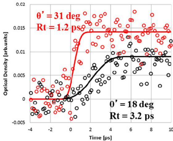
Figure 3: Rising behaviour of the optical absorption by hydrated electron measured at 800 nm.
