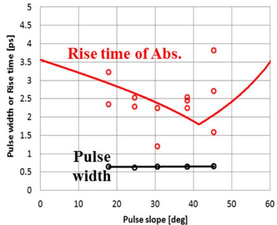
Figure 4: the angle of the electron beam pulse versus the pulse width and the rise time of absorption.
