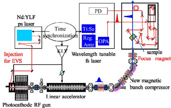
Figure 1: Pulse radiolysis system with the EVS method.
