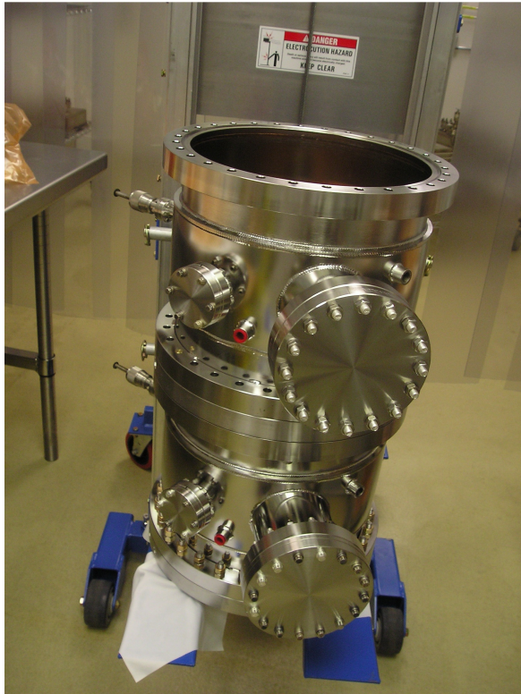
Figure 2: Clean room assembly of separator cavity.
