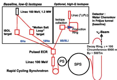
Figure 1: The CERN Beta Beam. The beta active isotopes are accelerated to the Decay Ring:  $^6\text{He}/^{18}\text{Ne}$  (low-Q) with a detector in Fréjus (baseline) and optionally  $^8\text{Li}/^8\text{B}$  (high-Q) with a detector at 700 km (Gran Sasso or Canfranc).
