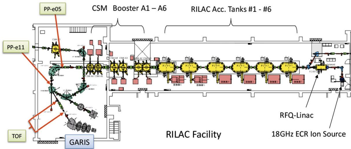
Figure 1: Layout of RILAC just after GARIS was installed, in 2002.
