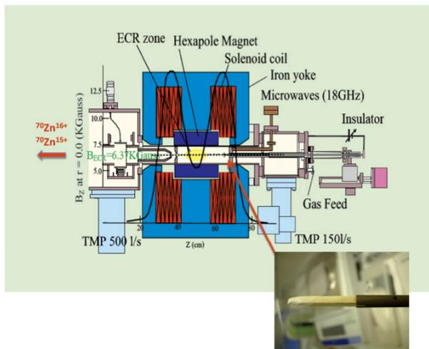
Figure 2: A cross-sectional view of 18GHz ECR Ion Source and Zn ceramic rod (photo).
