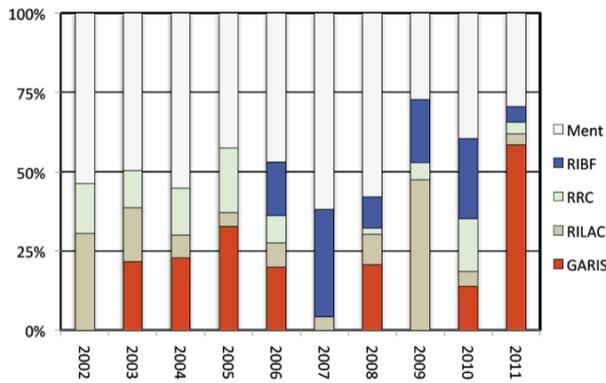
Figure 4: The operation statistics of RILAC, 2002 - 2011. In each year, 8760hr corresponds to 100%.
