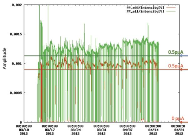
Figure 5: The 3<sup>rd</sup> harmonic signals from PP-e05(red curve) and PP-e11(green curve) measured from 14 March 2012 to 15 April 2012. Two calibration lines corresponding to 0.5 $\mu\text{A}$  for each probe are shown. Red line is for e05, and green one for e11.
