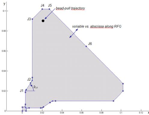
Figure 1: RFQ cross-section (x and y in meter units).
