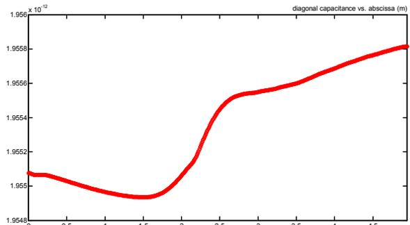
Figure 6: Parallel capacitance (F/m) vs. abscissa (m).
