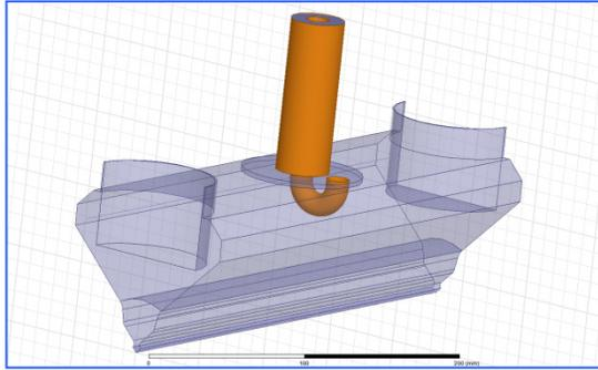
Figure 11: Coupling loop located between two tuners.
