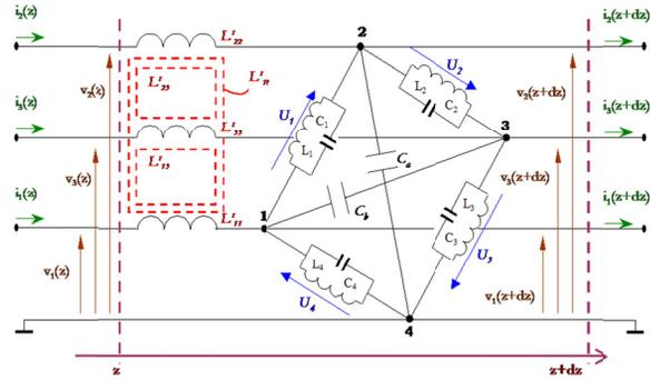
Figure 3: The 4-wire transmission line model (TLM).
