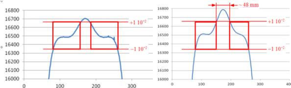
Figure 12:  $V/H_z$  perturbation induced by a loop in  $0^\circ$  (left) and  $45^\circ$  (right) position, and located between two tuners in +35 mm position, is  $< 1\%$  in red boxes.
