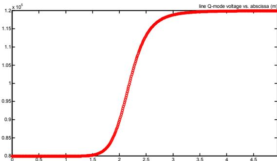
Figure 2: RFQ voltage profile (V) vs. abscissa (m).
