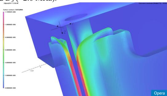
Figure 7: A view of E field amplitude at RFQ input.
