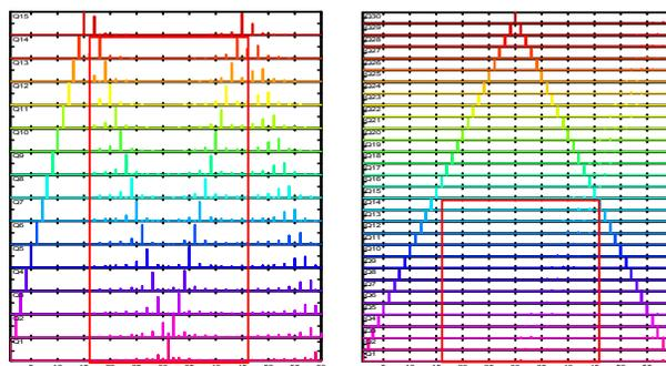
Figure 10: Left: spectral components of Q eigen-functions. Right: transmittance of reconstructing filter-bank. Spurious components in the red box are rejected.
