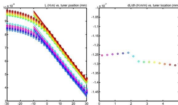
Figure 8: Left: 2D inductance vs. tuner position and tuner location (color-coded); right: inductance slope vs. tuner location (same color code).
