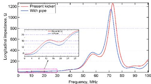
Figure 13: Impedance reduction at low frequency.
