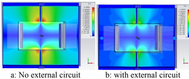
Figure 5: Induced magnetic flux in ferrite.
