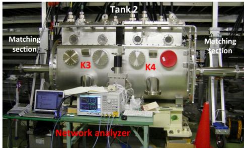
Figure 9: Impedance wire measurement setup (tank2).
