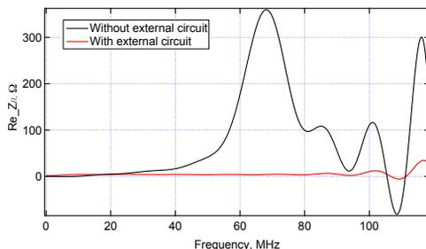
Figure 6: Comparison of coupling impedance with and without external circuit.
