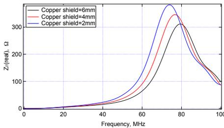
Figure 4: Coupling impedance with strip thickness.
