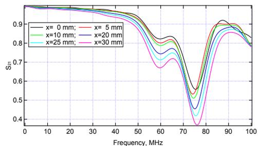
Figure 8: Transmission parameter  $S_{21}$  at different offset.
