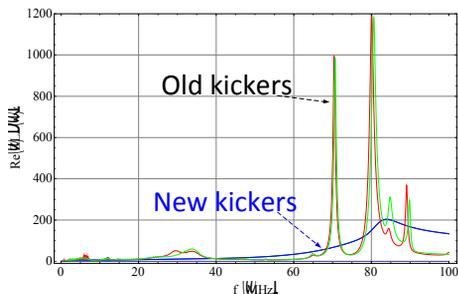
Figure 11: Comparison of impedance between old and new kickers.
