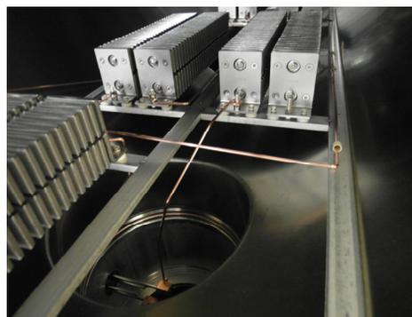
Figure 1: Major ionization beam loss has been caused by pressure bumps in the electrostatic injection septum. To enhance the pumping power and to speed up the recovery process, two sets of NEG panels have been installed in the electrostatic injection septum.
