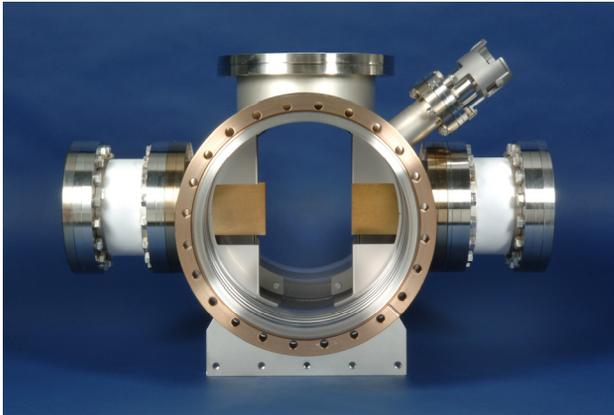
Figure 2: Low desorption charge scraper installed in the SIS18. Charge scrapers have been installed in all sections of SIS18, downstream each dipole pair. At these positions, stripped beam ions are well separated from the reference ions and can be scraped off without affecting the machine acceptance.
