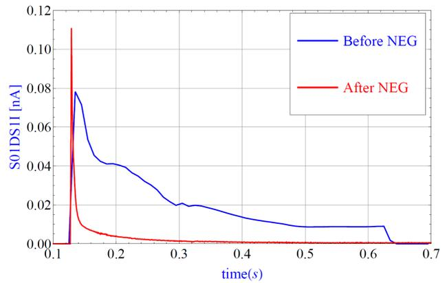
Figure 3: The electrical current measured on the charge scraper in section one has been significantly reduced by means of the NEG panels in the injection septum. This indicates that the pressure bump at injection and consequently the ionization beam loss in the injection section have been effectively removed.
