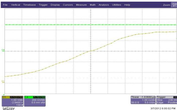
Figure 7: Jitter measurement at 50 kV, 1 Hz repetition rate.
