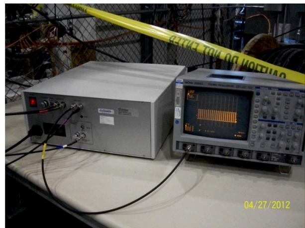
Figure 2: FID pulse generator under 50 kV, 1 kA, and 100 Hz test.
