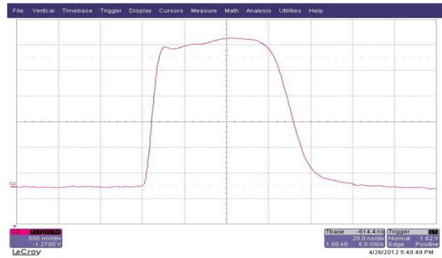
Figure 5: Load current waveform with 50 Ω oil cooled resistor stack and 250 feet of high voltage pulse transmission cable.
