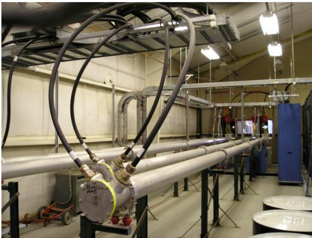
Figure 1: RHIC injection kicker Blumlein triaxial pulse generators.
