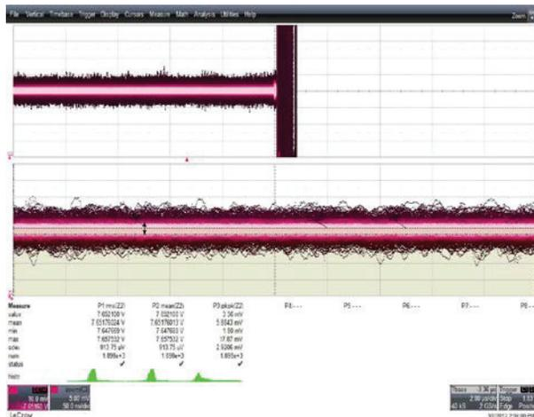
Figure 3: PFN voltage stability.
