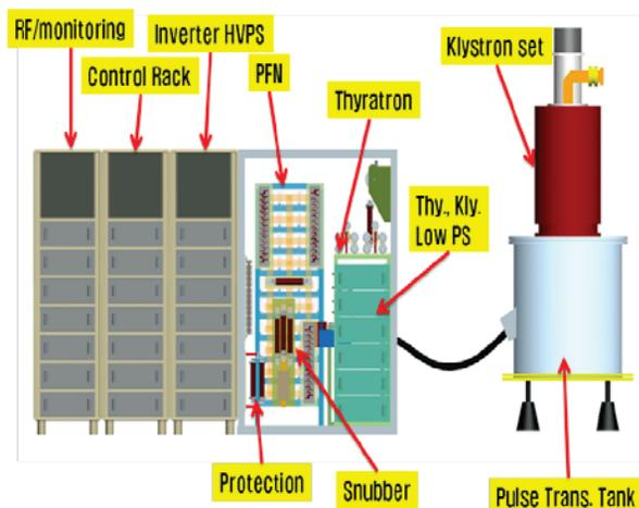
Figure 1: Configurations of the PLS-II modulator system.
