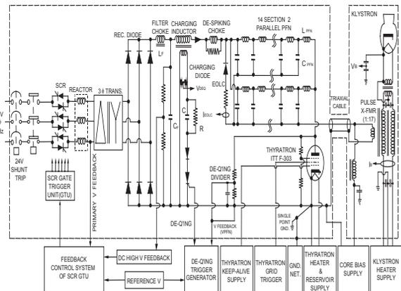
Figure 4: Schematic circuit diagram of the modulator.
