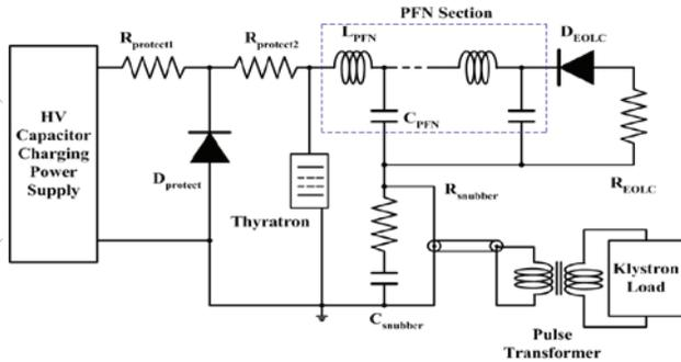
Figure 2: The schematic diagram of the PLS-II modulator.
