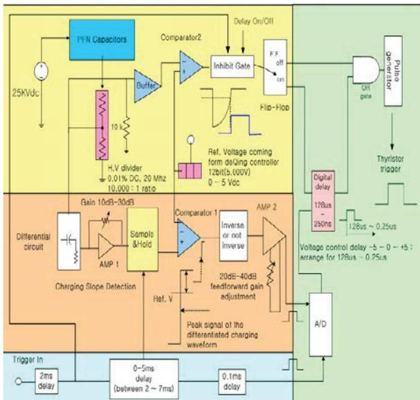
Figure 5: De-Qing block diagram.
