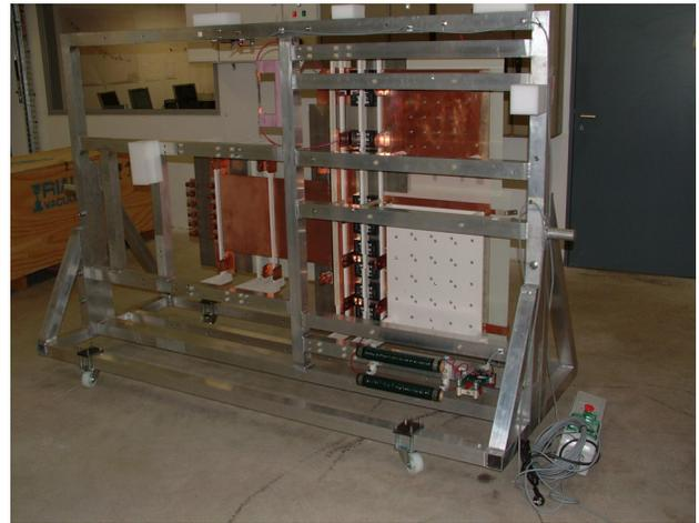
Figure 2: The prototype pulser during assembly.
