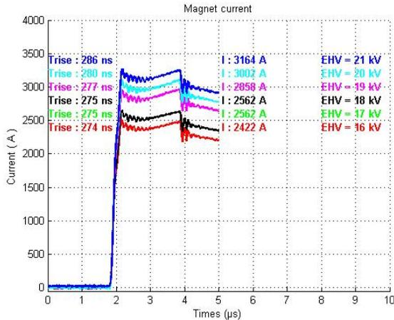
Figure 4:  $T_{rise}$  measurement for the extraction kicker.
