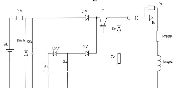
Figure 1: Kickers circuit schematics.
