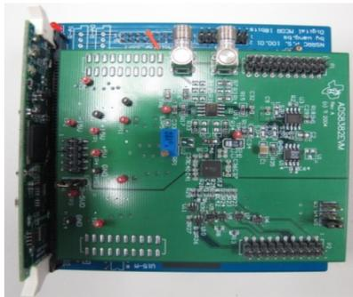
Figure 3: The picture of digital control card.
